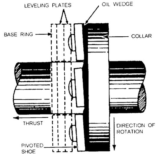
Figure 11-3.-Diagrammatic arrangement of a Kingsbury thrust bearing, showing oil film.
