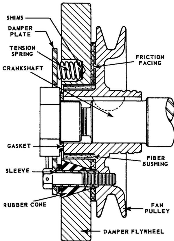
Figure 12-21.-Sectional view of a typical vibration damper.
