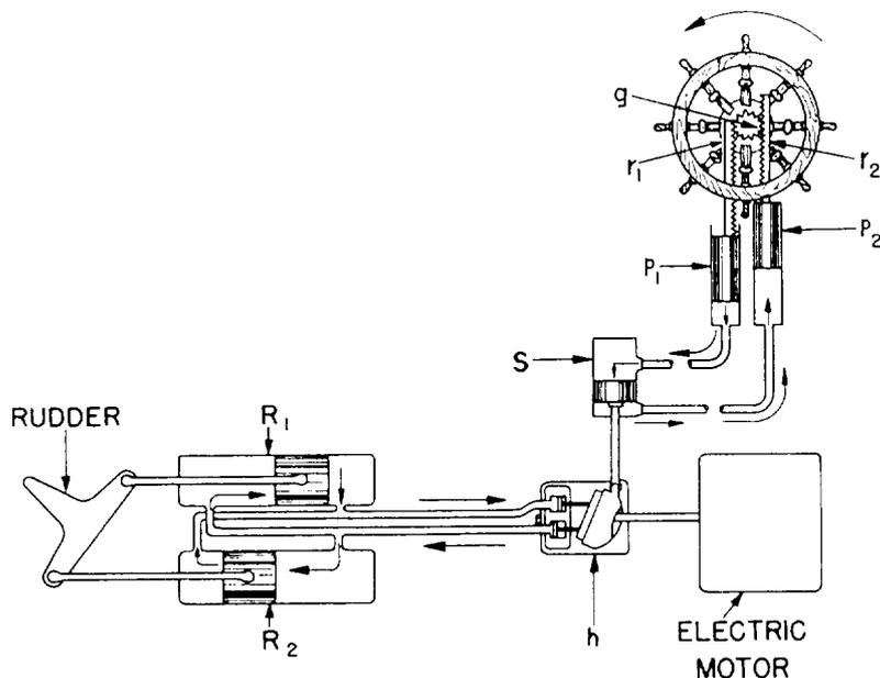
Figure 10-11.-Electrohydraulic steering mechanism.
