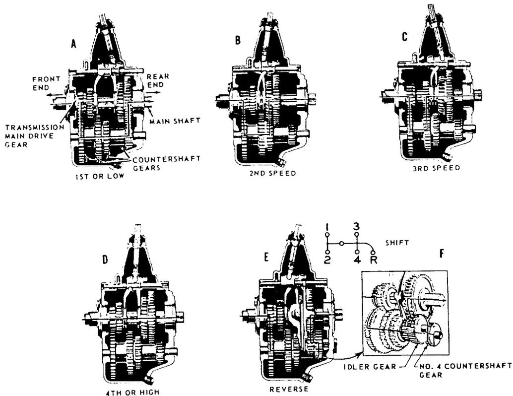
Figure 13-6.-Power flow through a four-speed transmission.
