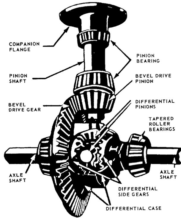
Figure 13-18.-Differential with part of case cut away.
