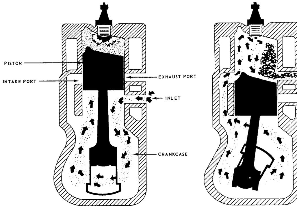
Figure 12-5.-Events in a two-cycle, internal combustion engine.
