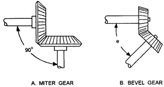
**Figure 6-5.—Bevel gears.**
