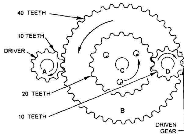
Figure 6-9.-Gears can change speed of applied motion.
