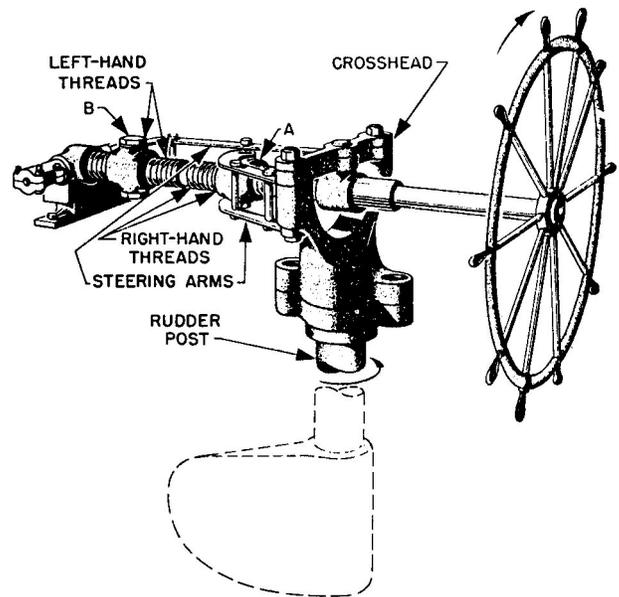
**Figure 5-8.—The screw gives a tremendous mechanical advantage.**
