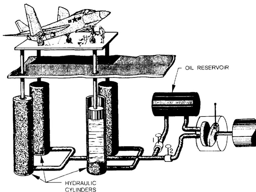
Figure 10-12.-Hydraulic lift.
