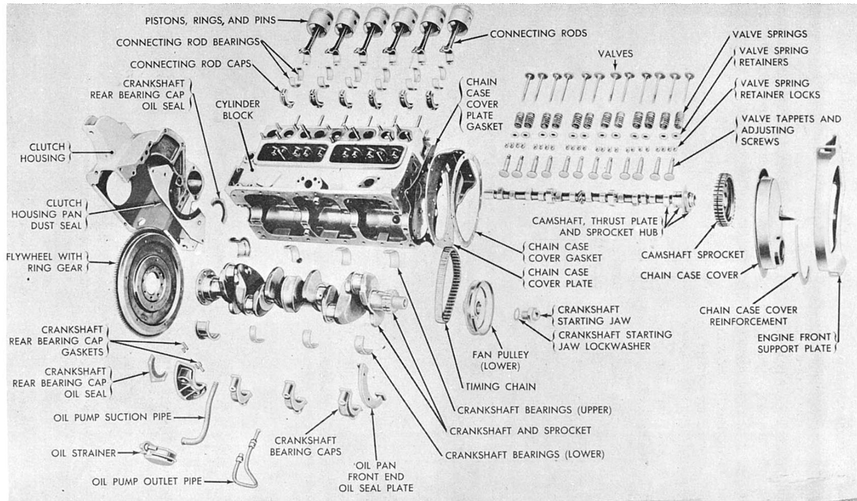
Figure 12-9.—Cylinder block and components.
