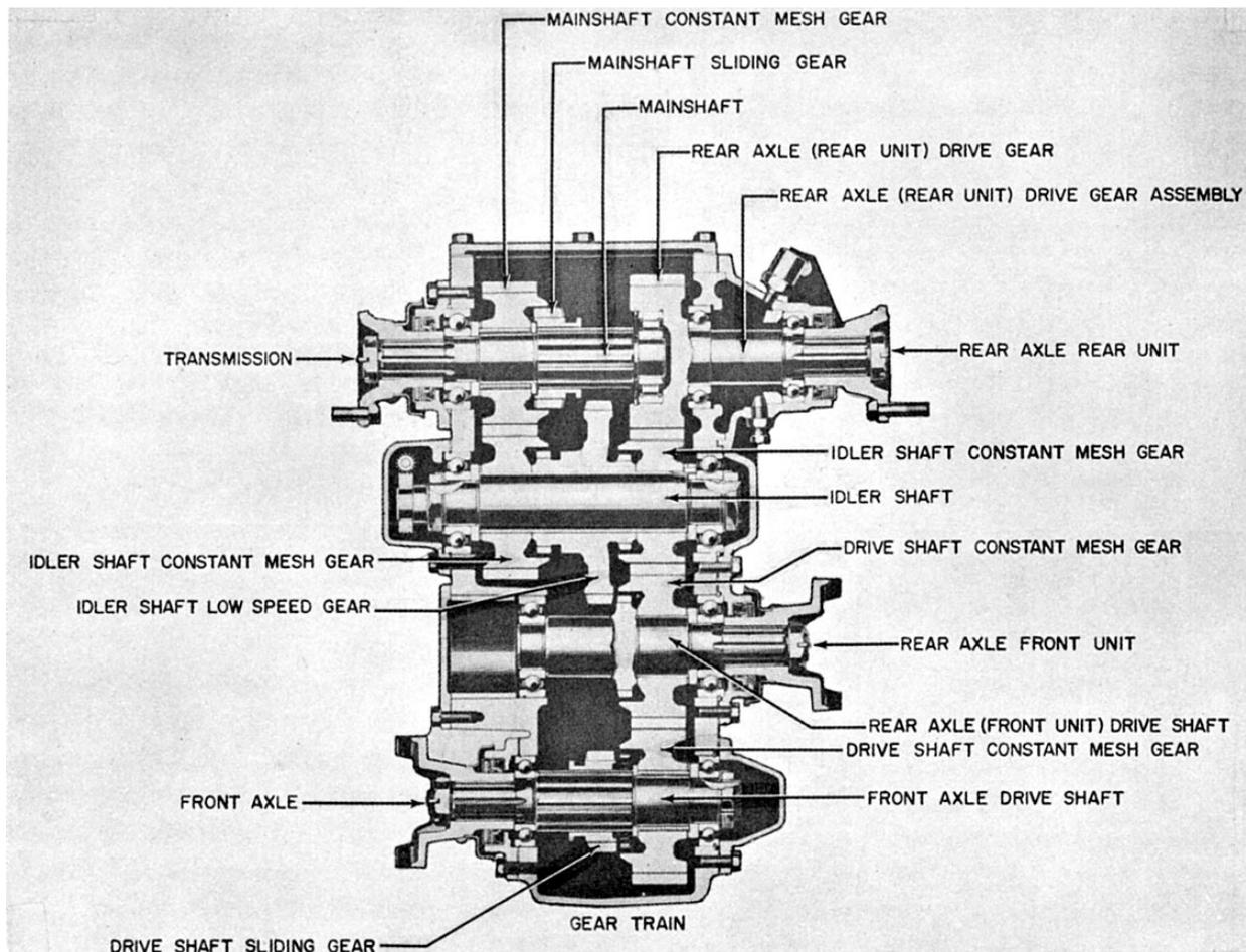
**Figure 13-14.-Cross section of a two-speed transfer case.**
