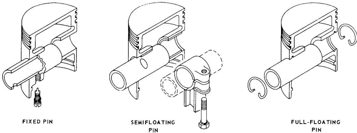
Figure 12-17.-Piston pin types.
