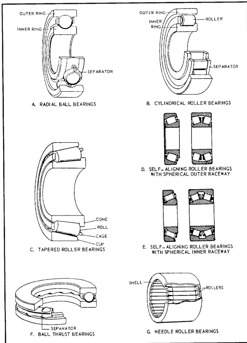
Figure 11-4. The seven basic types of antifrictional bearings.
