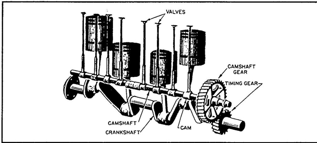
**Figure 6-13.—Automobile valve gear.**
