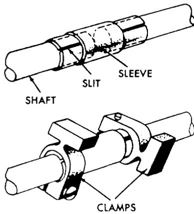
Figure 11-15.-Sleeve coupling.
