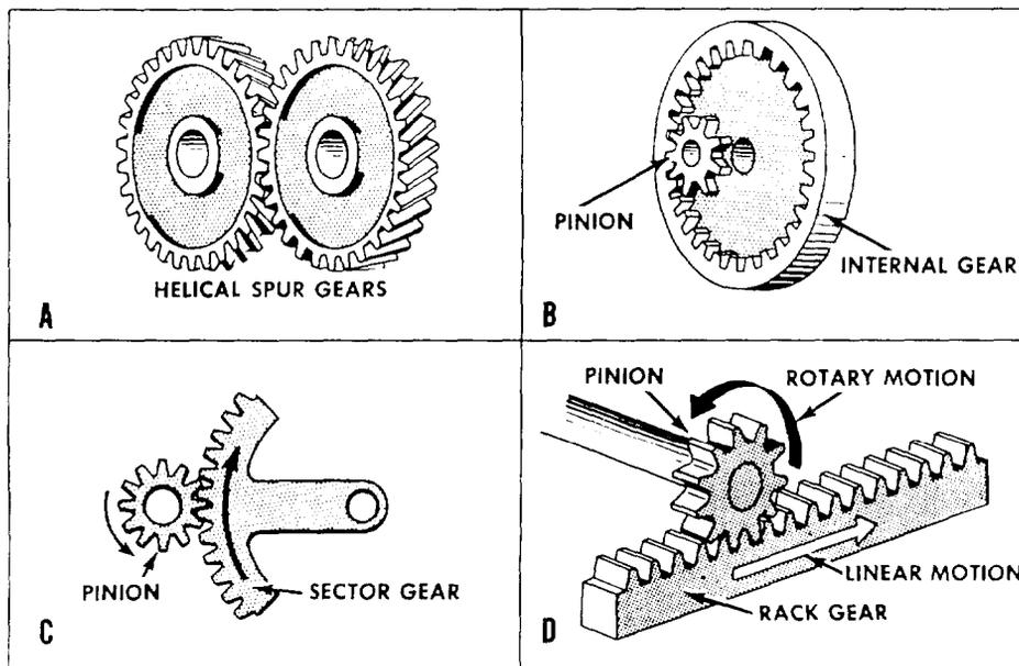
Figure 6-3.-Gear types.
