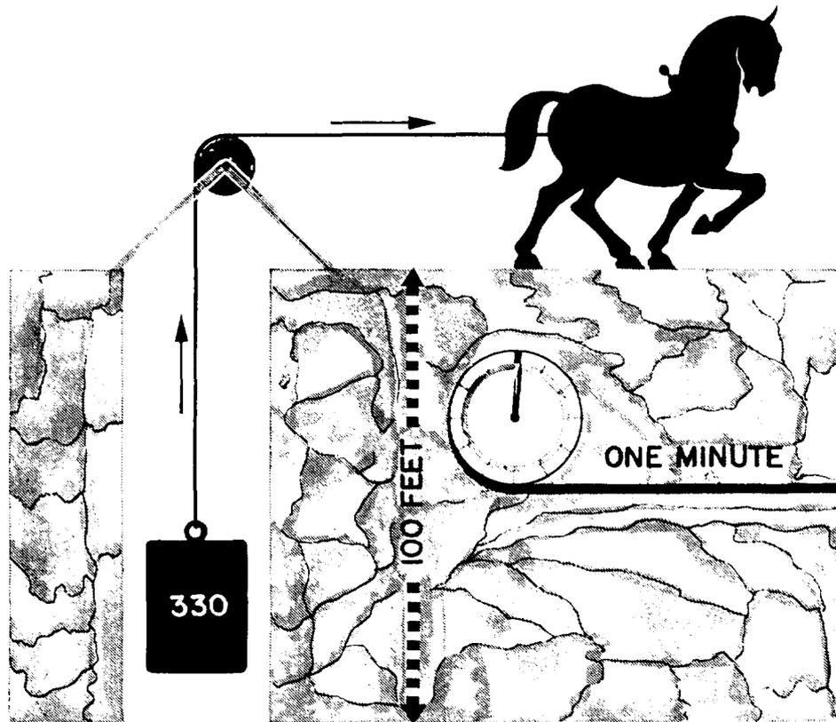
Figure 8-2.-One horsepower.
