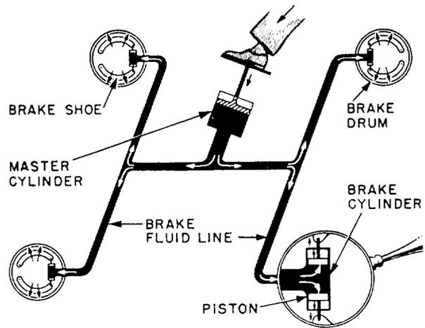
Figure 10-6.-Hydraulic brakes.
