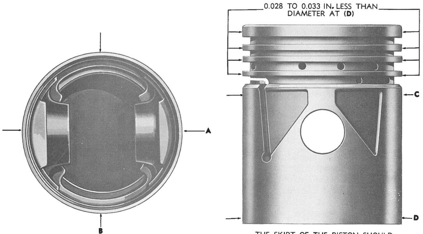
THE ELLIPTICAL SHAPE OF THE PISTON SKIRT SHOULD BE 0.010 TO 0.012 IN. LESS AT DIAMETER (A) THAN ACROSS THE THRUST FACES AT DIAMETER (B).
