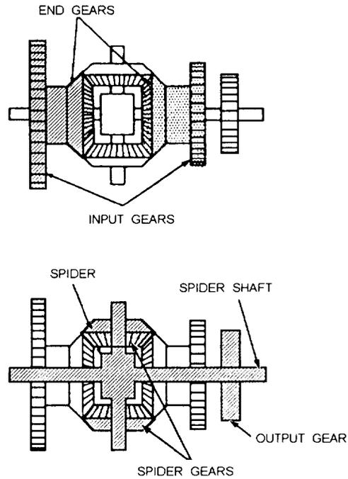
Figure 11-10.-The differential. End gears and spider arrangement.
