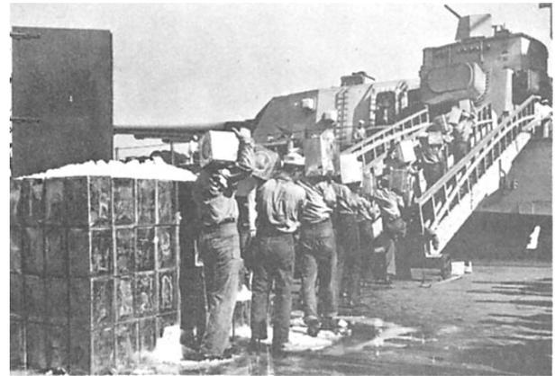
**Figure 4-3.—The gangplank is an inclined plane.**
