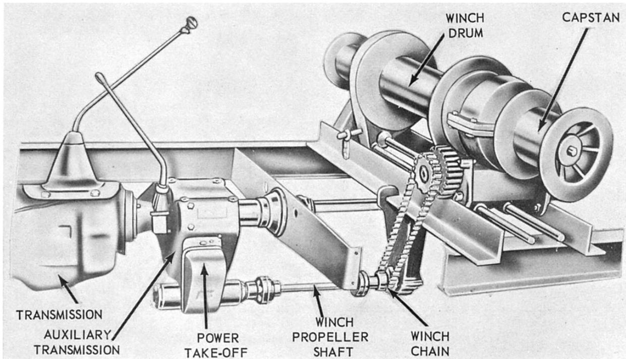
**Figure 13-12.—Auxiliary transmission power takeoff driving winch.**
