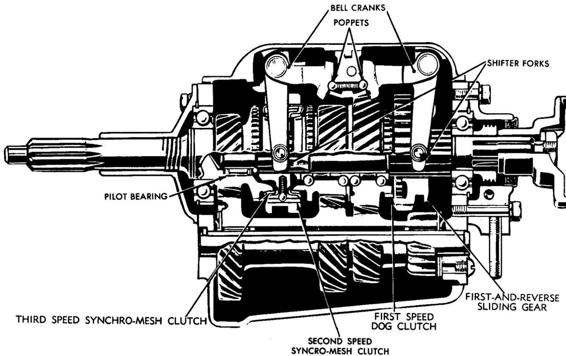
**Figure 13-10.-Synchromesh transmission arranged for steering column control.**
