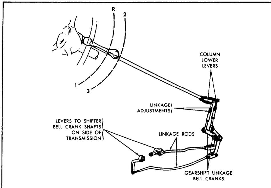
Figure 13-11.-Steering column transmission control lever and linkage.
