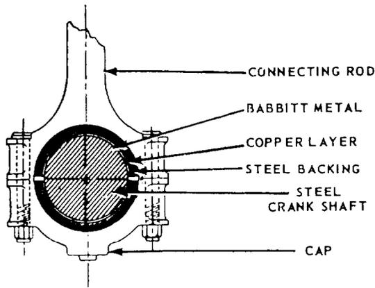
Figure 11-1.-Babbitt-lined bearing in which steel shaft revolves.
