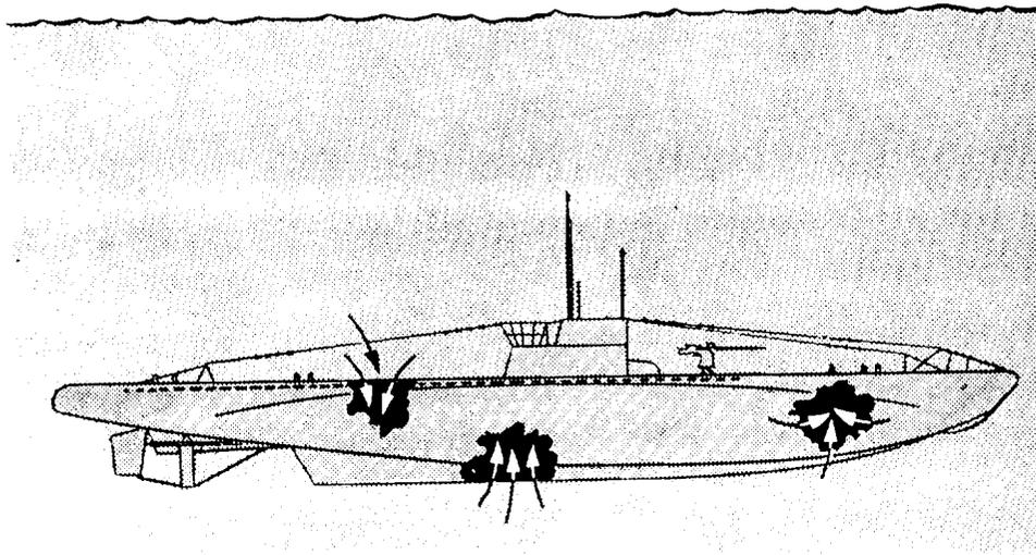
Figure 9-3.-Fluids exert pressure in all directions.
