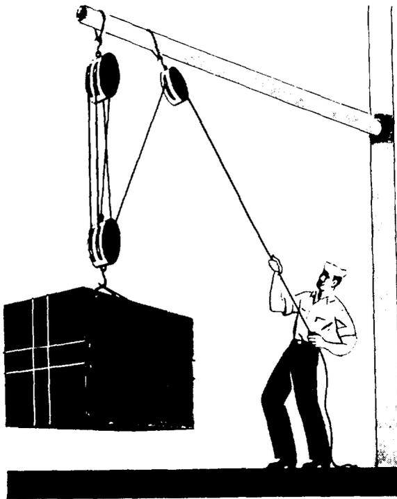
Figure 7-5.—A block and tackle makes work easier.
